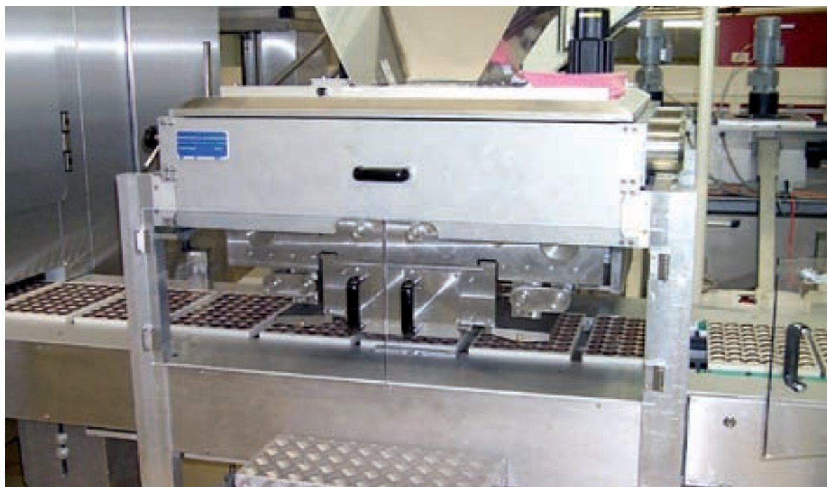
The RFID monitoring system instantly emits an alarm if inserted molds are not suitable for the production process underway
